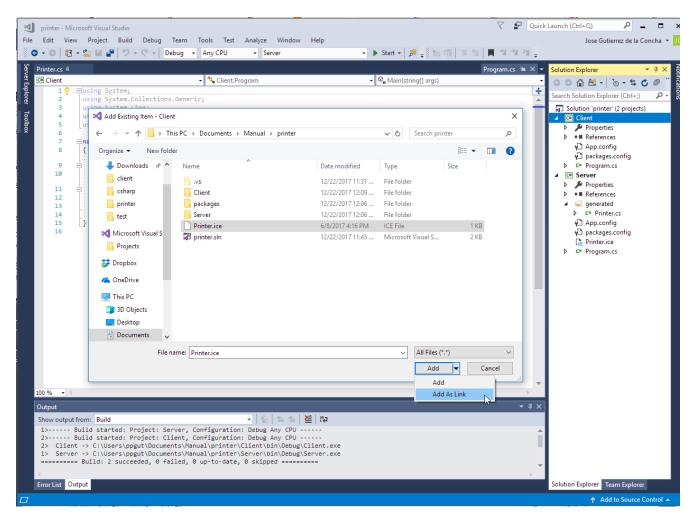
If the Ice Builder for Visual Studio is installed, it immediately generates the file generated\Printer.cs from Printer.ice unless you disabled au tomatic building in the Ice Builder.
